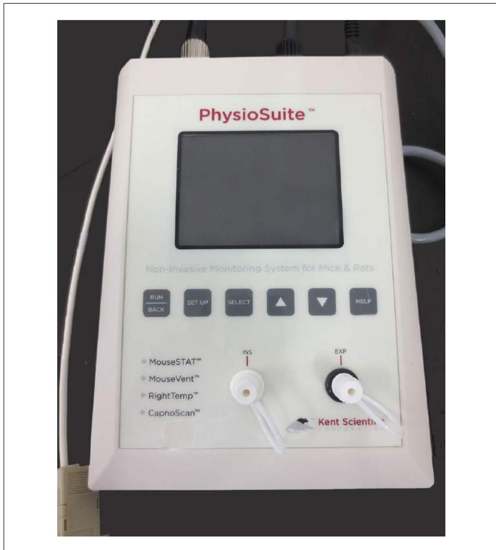
**Figure 4** The PhysioSuite (Kent Scientific) is an example of a commercially available tool for mice that provides pulse oximetry, heart rate, ventilator control, capnography (end tidal CO<sub>2</sub>), and body temperature.
